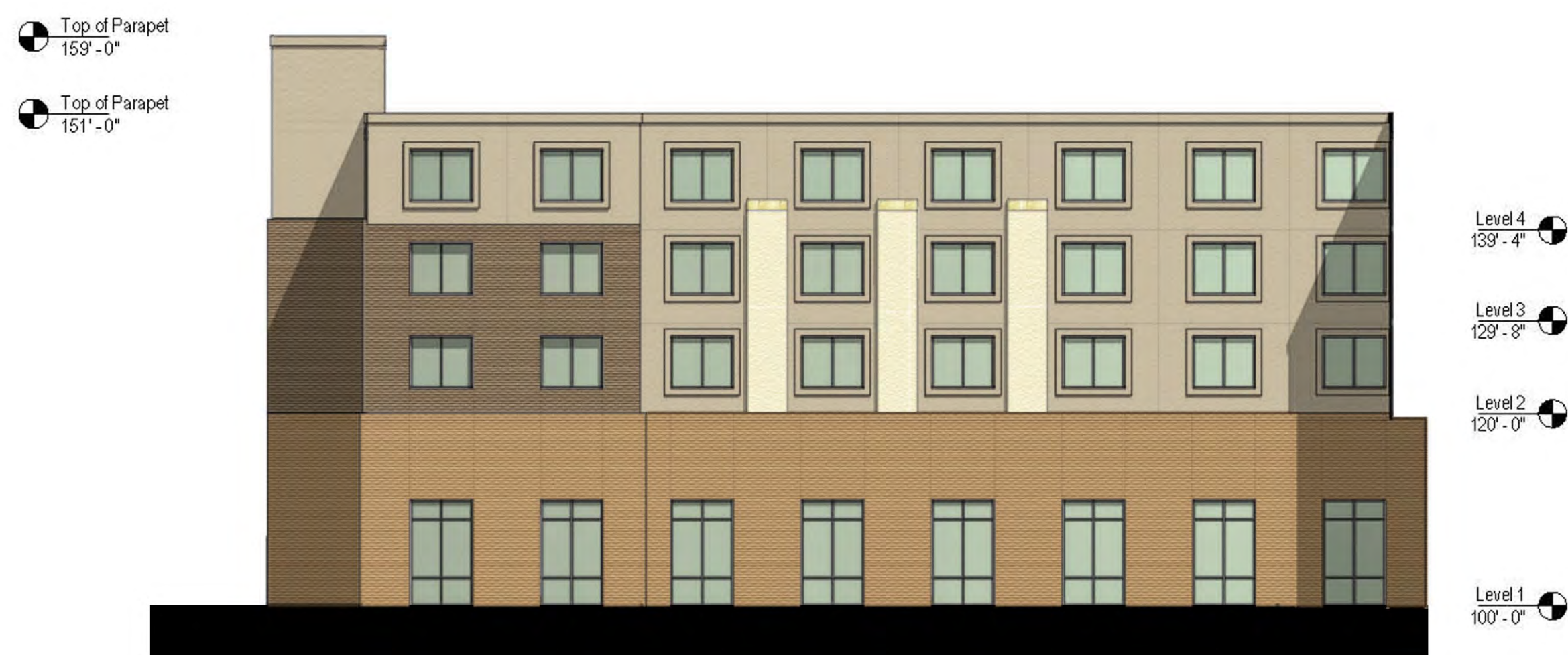
east elevation 2 53.2% masonry
