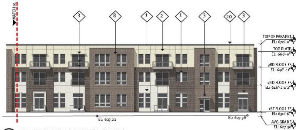
02 BLOCK B NORTH ELEVATION (HOWELL ST)
