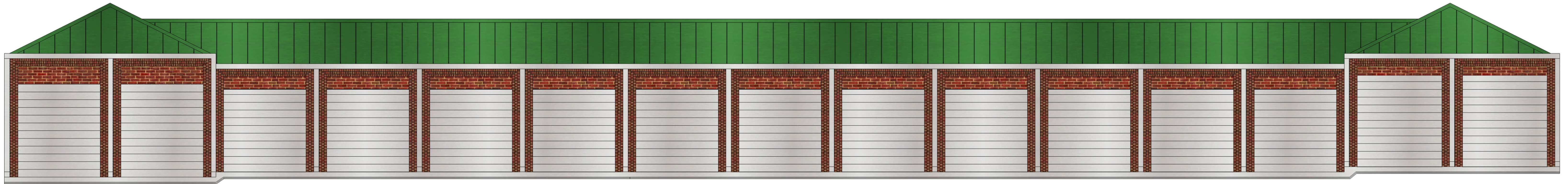
Buildings # 5, 7, 9 & 11 South Elevation 100% Masonry (less Doors and Downspouts)
