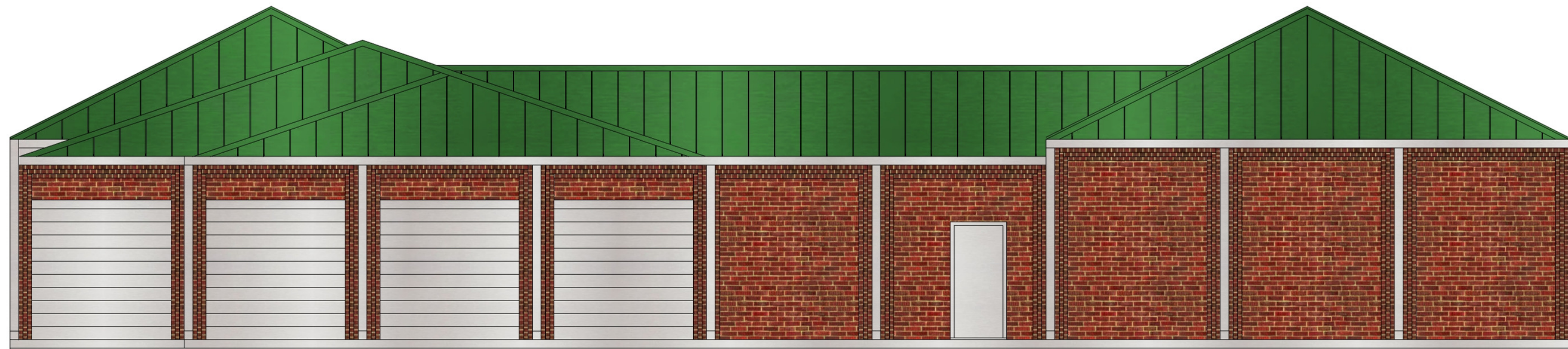
Building # 2 West Elevation 100% Masonry (less Doors and Downspouts)
