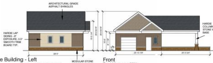
Maintenance Building - Left Total Masonry: 53% Stone: 21% Brick: 32% Lap: 38% Trim: 9%
