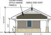
Mail Kiosk - Side 1 Total Masonry: 63% Stone: 27% Brick: 36% Shake: 32% Trim: 5%
