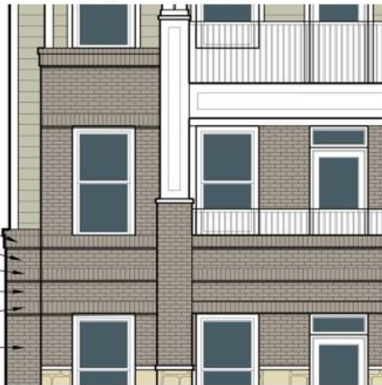
Brick Pattern Detail - Typ. at all buildings where indicated
