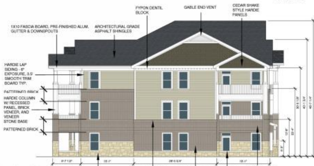
2. Building Type II - 3 Story - Side
