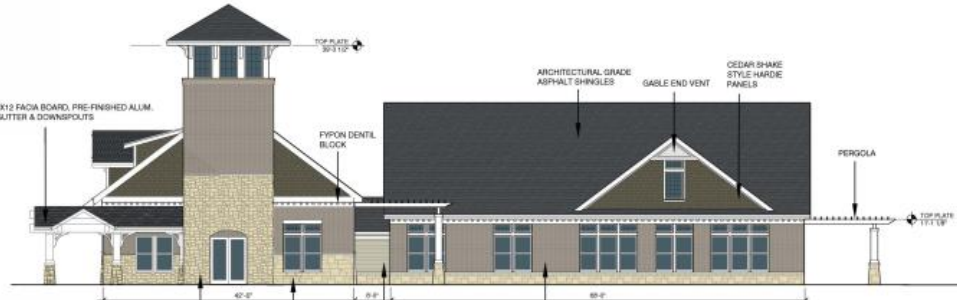
4. Clubhouse - South Total Masonry: 69% Brick: 68% Stone: 32% Lap: 2% Shake: 25% Trim: 4%
