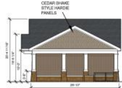
Right Total Masonry: 66% Stone: 20% Brick: 46% Shake: 28% Trim: 6%
