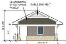
Mail Kiosk - Side 2 Total Masonry: 63% Stone: 27% Brick: 36% Shake: 32% Trim: 5%
