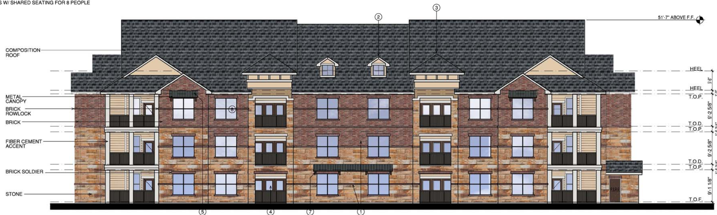
2 BUILDING 'C' REAR NORTH ELEVATION (BLDG. #4) SCALE 1/8"=1'-0"
