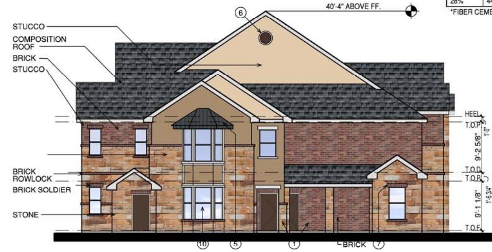
3 BUILDING 'D' END EAST ELEVATION (BLDG. #3) SCALE 1/8"=1'-0"
