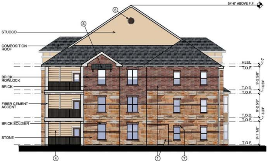
4 BUILDING 'F' END EAST ELEVATION (BLDG. #9) SCALE 3/32"=1'-0"
