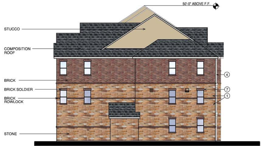
3 BUILDING 'A' END EAST ELEVATION (BLDG. #6) SCALE 1/8"=1'-0"
