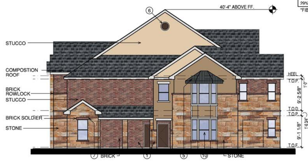
4 BUILDING 'D' END WEST ELEVATION (BLDG. #3) SCALE 1/8"=1'-0"
