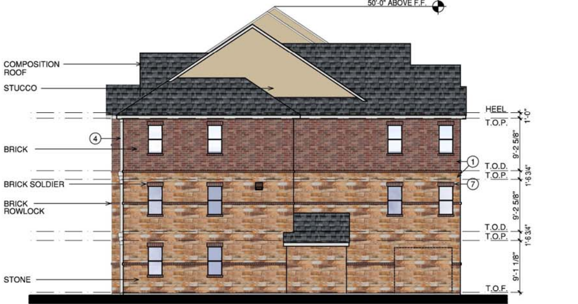
4 BUILDING 'A' END SOUTH ELEVATION (BLDG. #1) SCALE 1/8"=1'-0"
