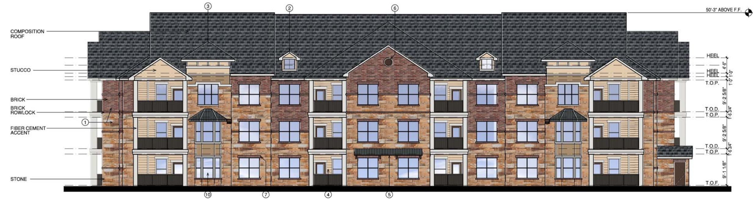
2 BUILDING 'B' REAR NORTH ELEVATION (BLDG. #8) SCALE 1/8"=1'-0"
