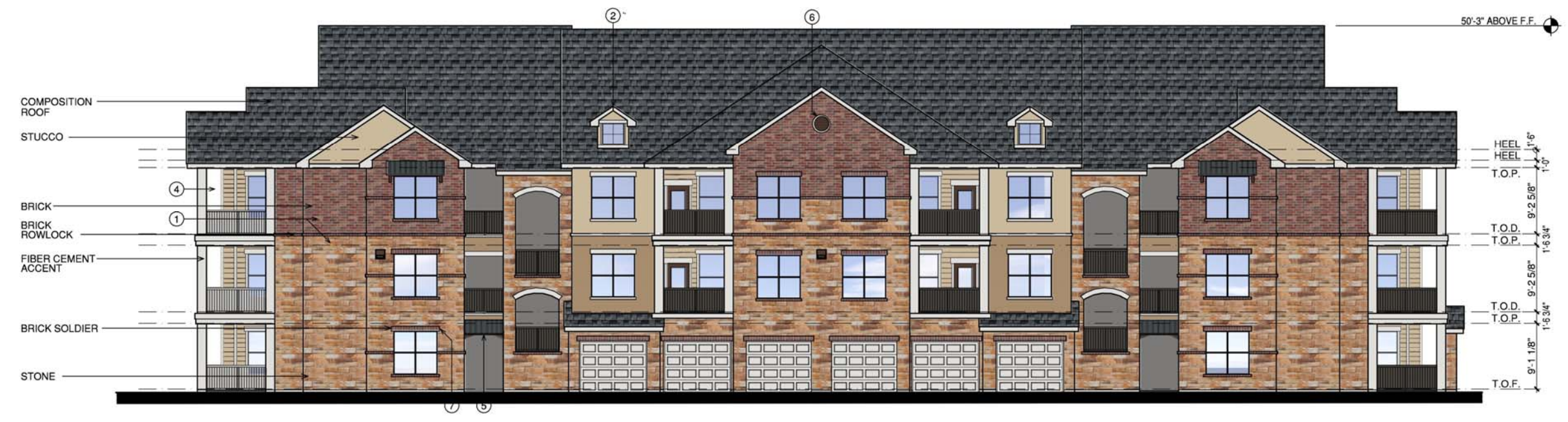
1 BUILDING 'B' FRONT EAST ELEVATION (BLDG. #5) SCALE 1/8"=1'-0"
