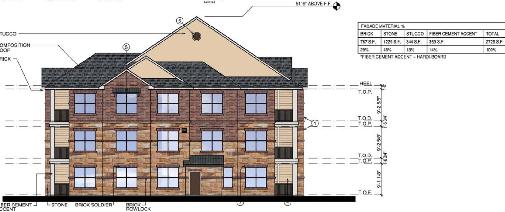
4 BUILDING 'C1' END EAST ELEVATION (BLDG. #10) SCALE 1/8"=1'-0"
