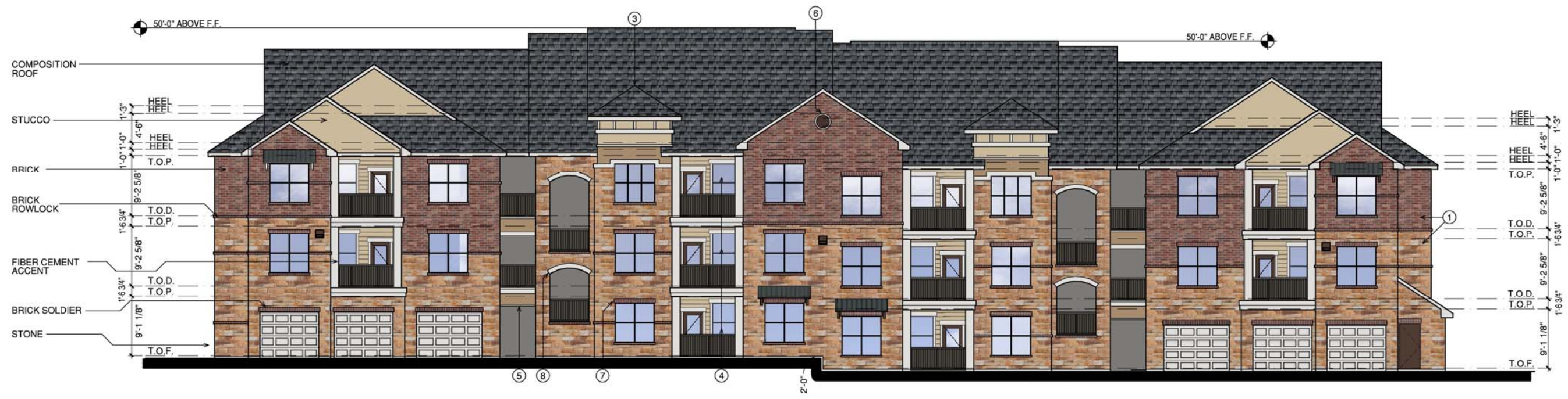
1 BUILDING 'A' FRONT SOUTH ELEVATION (BLDG. #6) SCALE 1/8"=1'-0"
