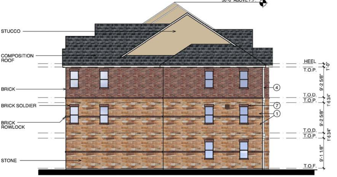
3 BUILDING 'A' END NORTH ELEVATION (BLDG. #1) SCALE 1/8"=1'-0"
