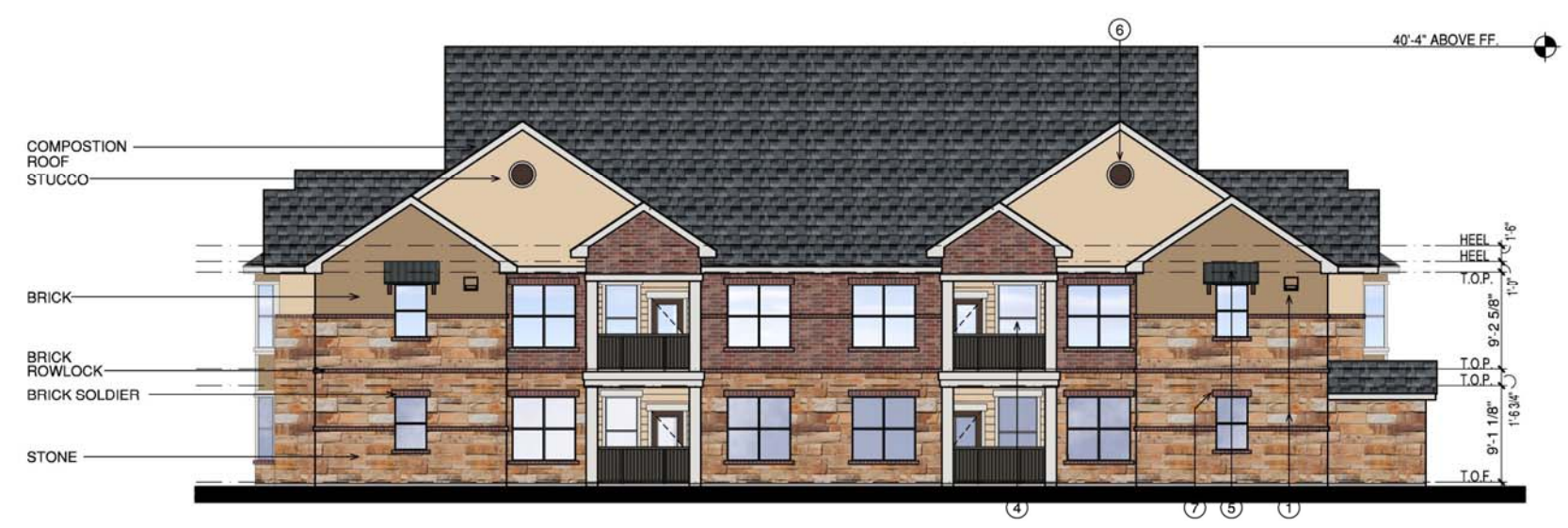
2 BUILDING 'D' REAR SOUTH ELEVATION (BLDG. #3) SCALE 1/8"=1'-0"
