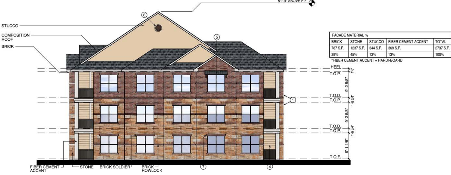
3 BUILDING 'C1' END WEST ELEVATION (BLDGS. #10) SCALE 1/8"=1'-0"
