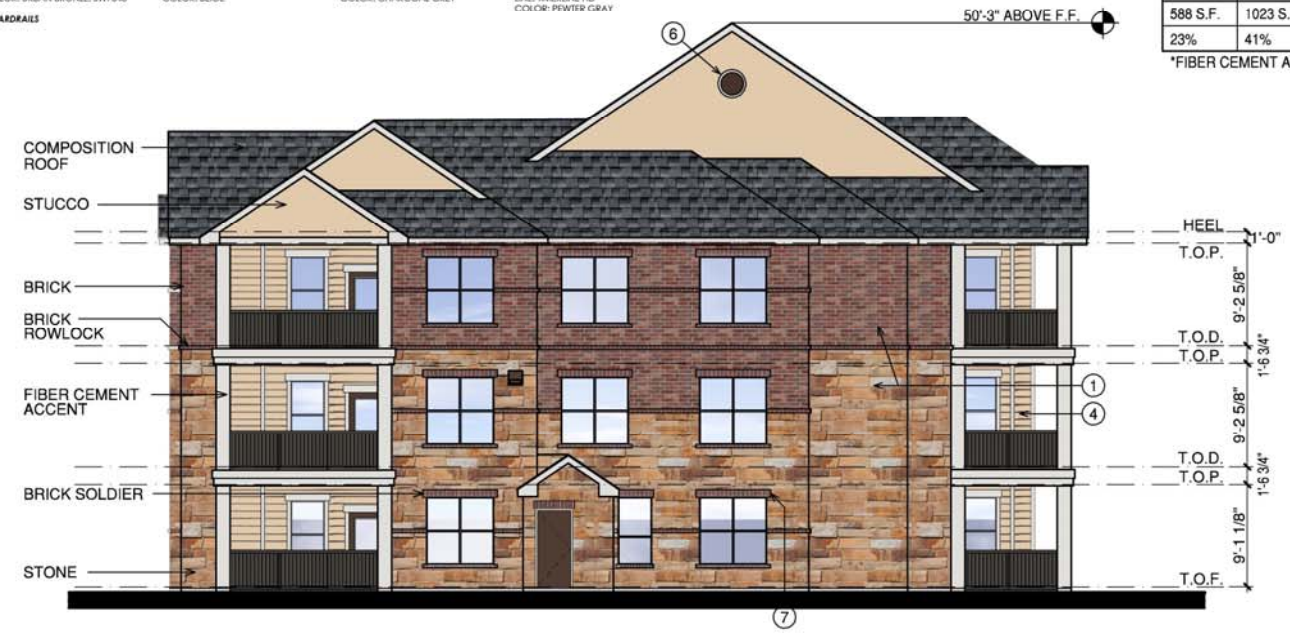
4 BUILDING 'B' END NORTH ELEVATION (BLDG. #5) SCALE 1/8"=1'-0"
