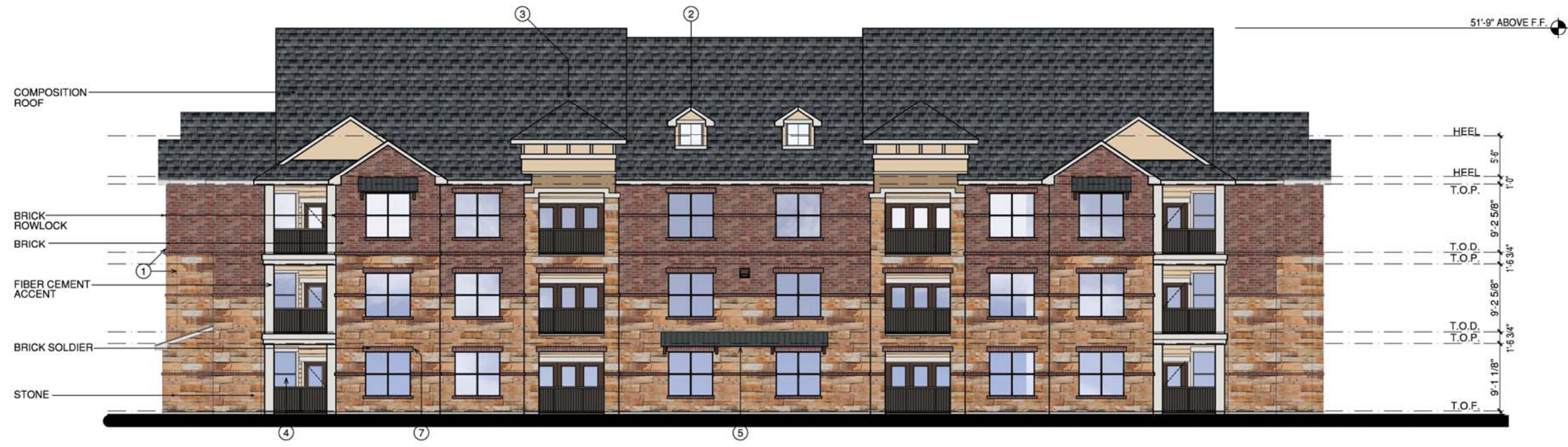
2 BUILDING 'C1' REAR NORTH ELEVATION (BLDGS. #10) SCALE 1/8"=1'-0"
