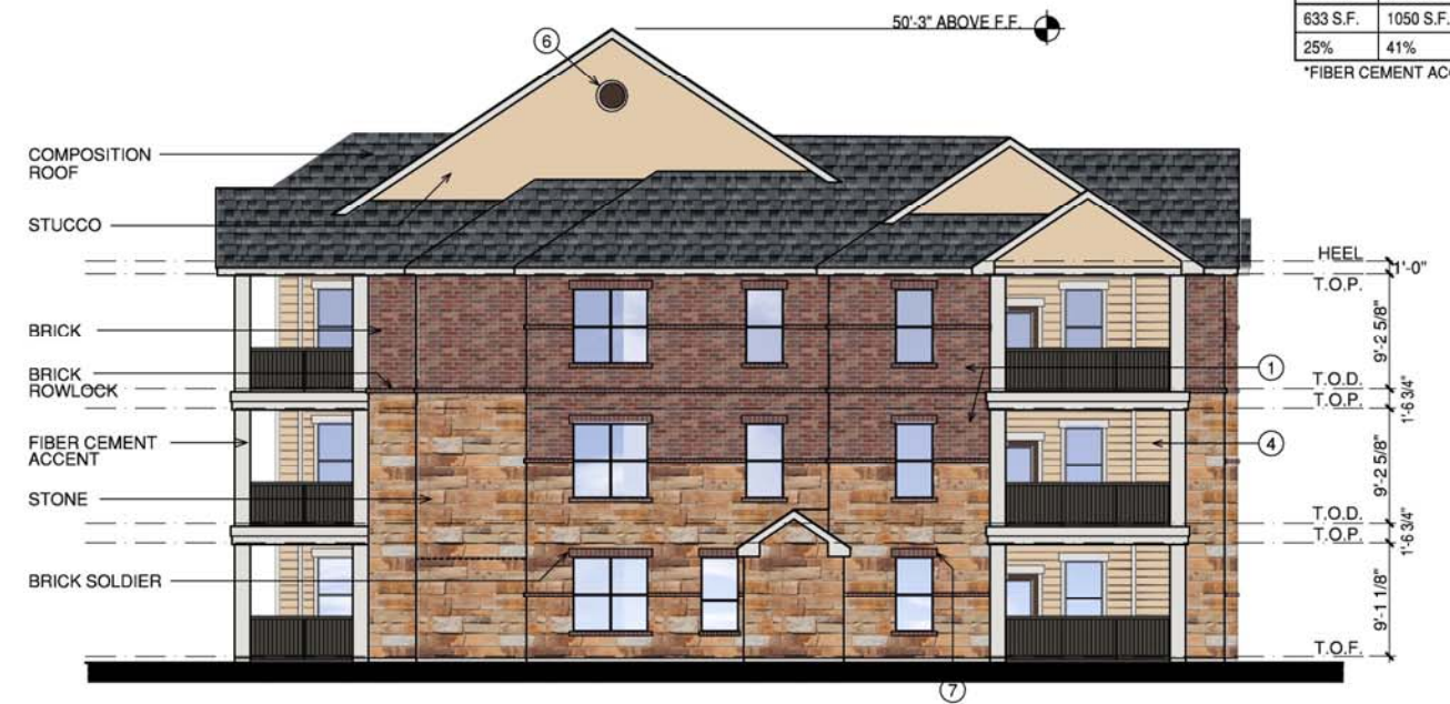
3 BUILDING 'B' END WEST ELEVATION (BLDG. #8) SCALE 1/8"=1'-0"
