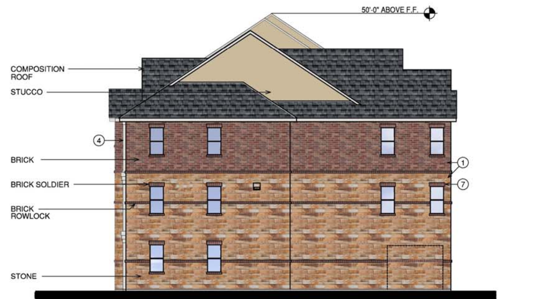
4 BUILDING 'A' END WEST ELEVATION (BLDG. #6) SCALE 1/8"=1'-0"
