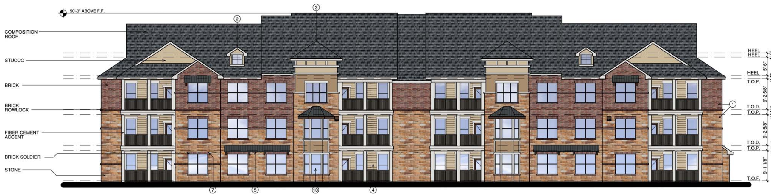
2 BUILDING 'A' REAR WEST ELEVATION (BLDG. #1) SCALE 1/8"=1'-0"
