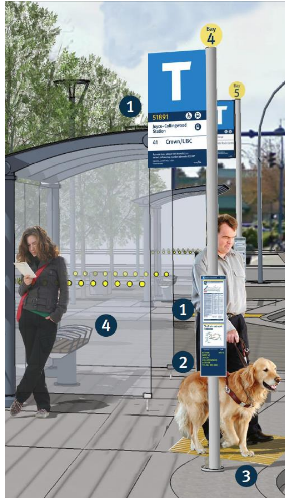
(C) An example of signage [1], route information [2], curb cuts [3], and shelter [4]
