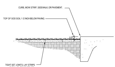
SOD INSTALLATION AT PAVEMENT/ CURB
