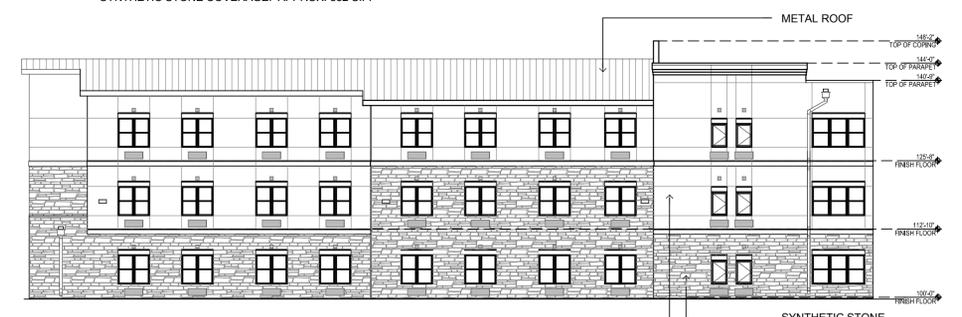
**B4 BUILDING B - WEST ELEVATION**
