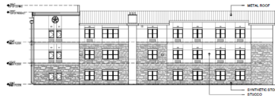
B1 BUILDING B - EAST ELEVATION
