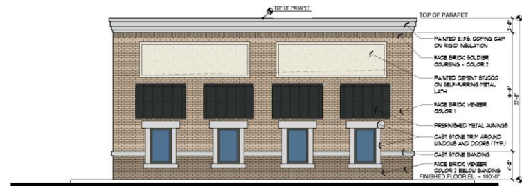
② SOUTH ELEVATION SCALE: 3/16" = 1'-0" EXT-EL01.DWG
