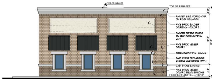
③ NORTH ELEVATION SCALE: 3/16" = 1'-0" EXT-EL01.DWG
