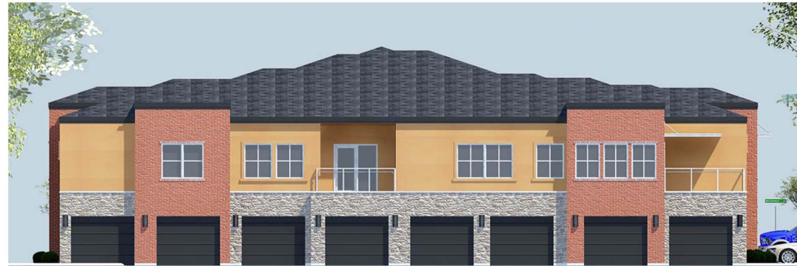
East Elevation - 60% Masonry (34% Brick, 26% Stone, 40% Stucco)
