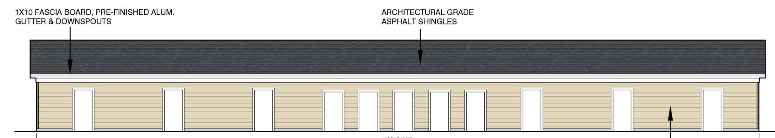
Storage Rear Masonry (Brick): 2% Lap: 94% Trim 4%
