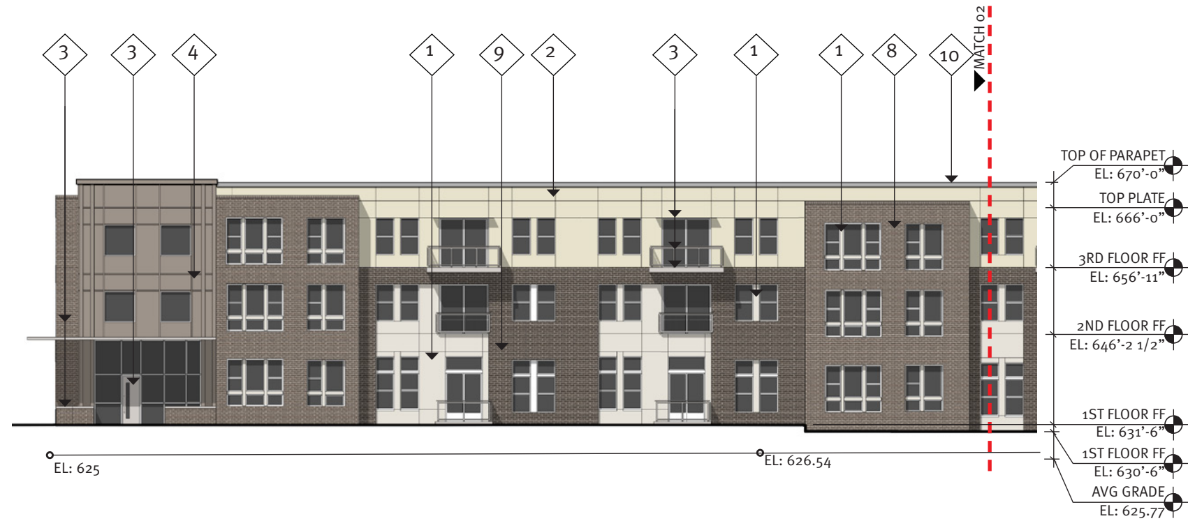
01 BLOCK B NORTH ELEVATION (HOWELL ST)
