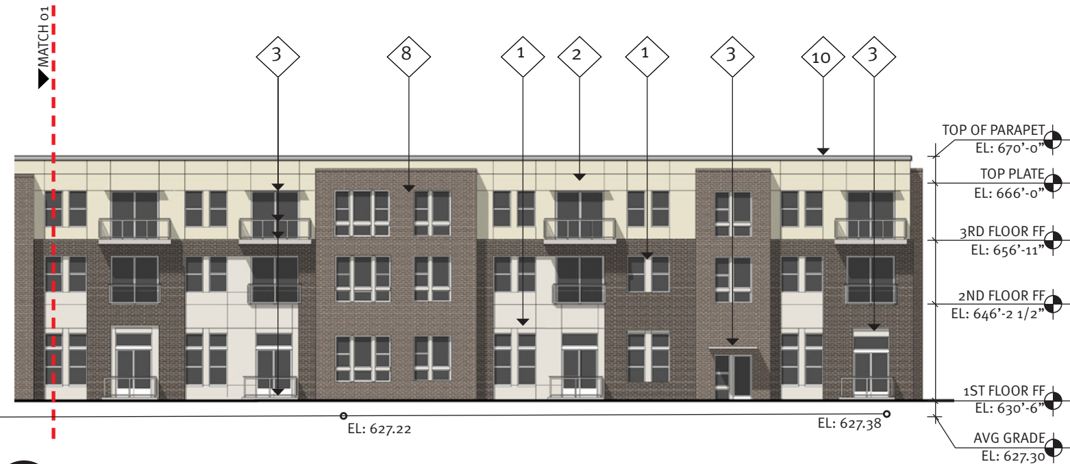
02 BLOCK B NORTH ELEVATION (HOWELL ST)
