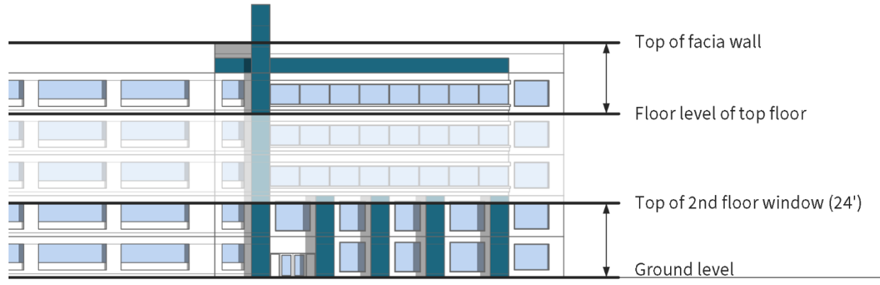
Figure 134-5: Permitted Sign Location
