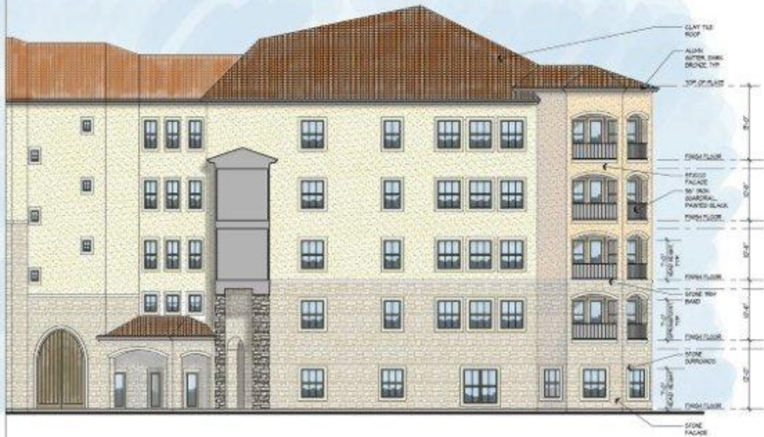
02 South East Elevation SCALE: 1/8" = 1'-0"
