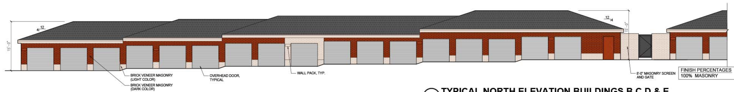
03 TYPICAL NORTH ELEVATION BUILDINGS B,C,D,& E SCALE: 1/8"=1'-0" SHOWN BUILDING B (C,D, & E SIMILAR VARIES WITH SLOPE)
