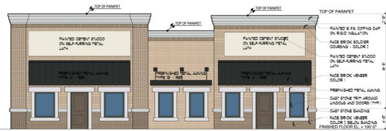
② EAST ELEVATION - FACING STREET SCALE: 3/16" = 1'-0" EXT-EL01.DWG
