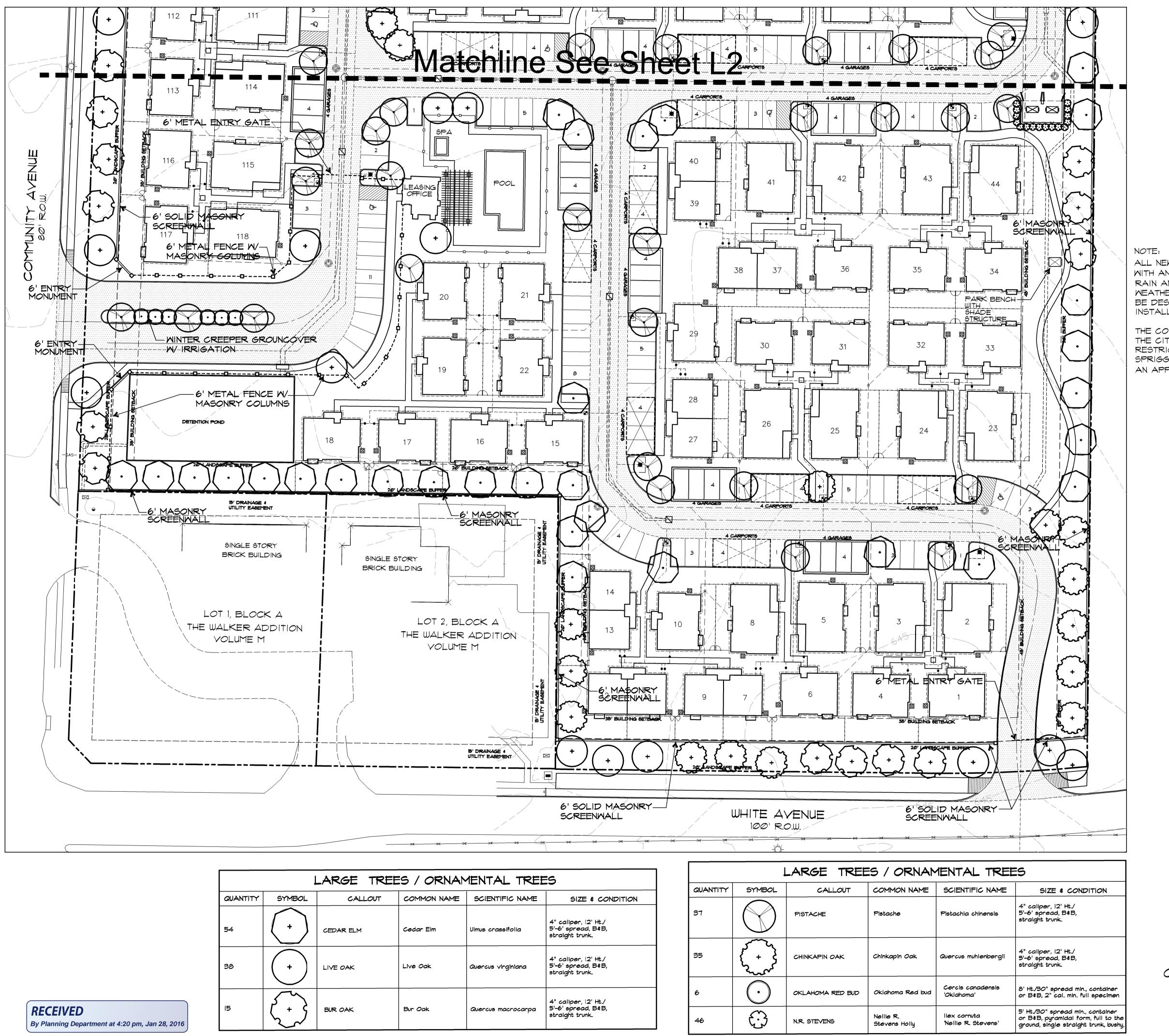
ALL NEW REQUIRED LANDSCAPE AREAS SHALL BE PROVIDED WITH AN AUTOMATIC UNDERGROUND IRRIGATION SYSTEM WITH RAIN AND FREEZE SENSORS, AND EVAPOTRANSPIRATION (ET) MEATHER BASED CONTROLLERS. AND SAID IRRIGATION SHALL BE DESIGNED BY A QAULIFIED PROFFESSIONAL AND INSTALLED BY A LICENSED IRRIGATOR.
