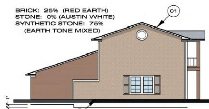
BUILDING #9 - SOUTH ELEVATION
