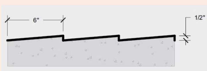
SHIPLAP WOOD CONCRETE FORMLINER PATTERN
