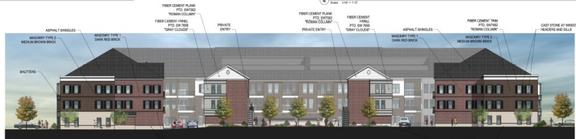
VIEW EAST THROUGH COURTYARD Scale: 1/16" = 1'-0"
