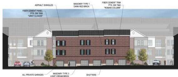
3 BAY CARRIAGE HOUSE WEST ELEVATION Scale: 1/8" = 1'-0"
