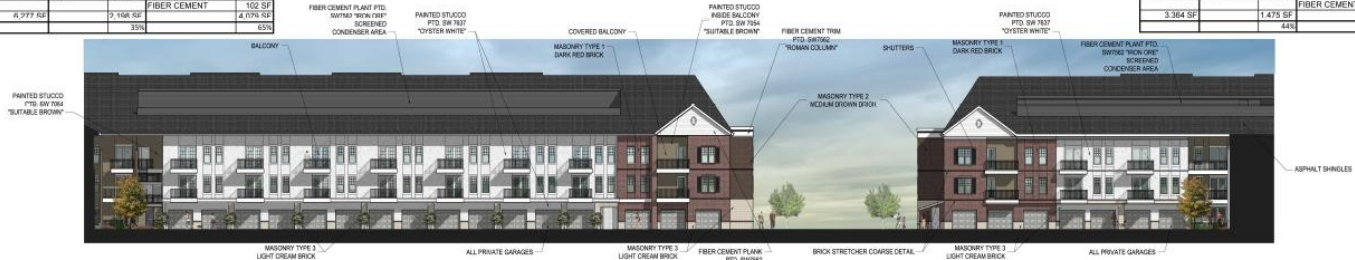
4 BUILDING B - NORTH COURTYARD ELEVATION Scale: 1/8" = 1'-0"
