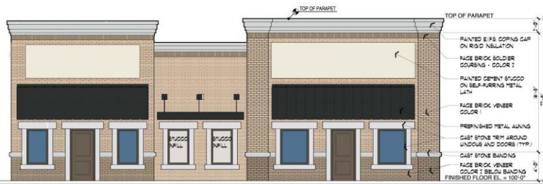
④ WEST ELEVATION - FACING PARKING SCALE: 3/16" = 1'-0" EXT-EL01.DWG
