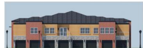
North Elevation - 63% Masonry (36% Brick, 27% Stone, 37% Stucco)
