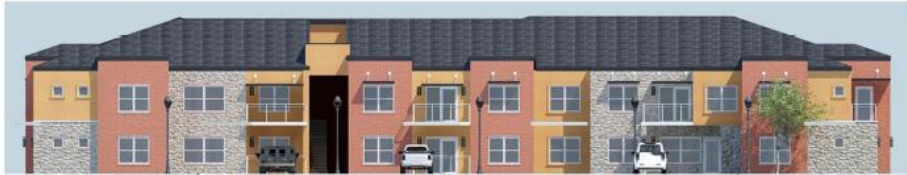
South Elevation - 69% Masonry (39% Brick, 30% Stone, 31% Stucco)
