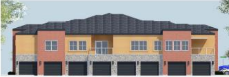
East Elevation - 60% Masonry (34% Brick, 26% Stone, 40% Stucco)
