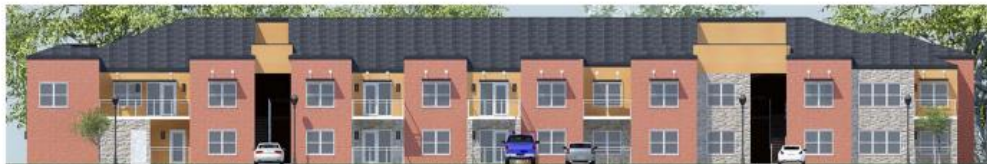
East Elevation - 79% Masonry (58% Brick, 19% Stone, 21% Stucco)
