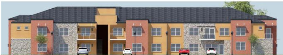
North Elevation - 61% Masonry (31% Brick, 30% Stone, 39% Stucco)
