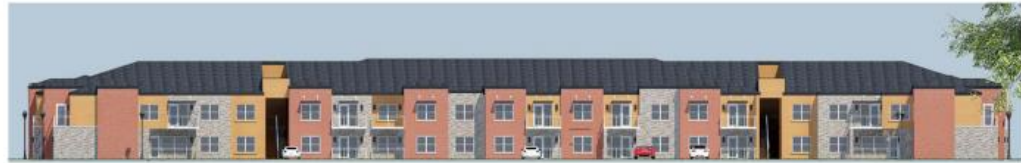
East Elevation - 80% Masonry (40% Brick, 40% Stone, 20% Stucco)
