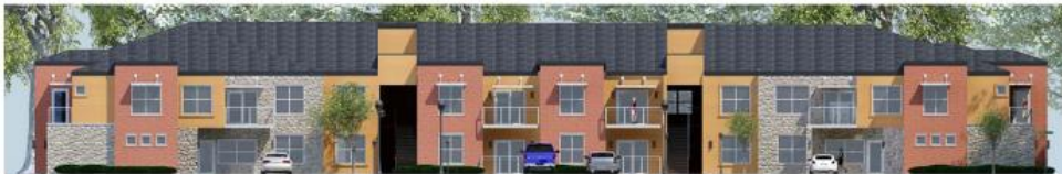
North Elevation - 65% Masonry (36% Brick, 29% Stone, 35% Stucco)
