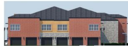
North Elevation - 86% Masonry (74% Brick, 12% Stone, 14% Stucco)
