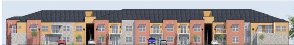
South Elevation - 74% Masonry (46% Brick, 34% Stone, 26% Stucco)
