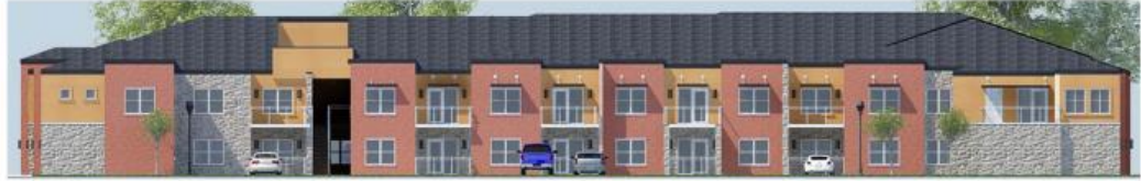
South Elevation - 79% Masonry (45% Brick, 34% Stone, 21% Stucco)
