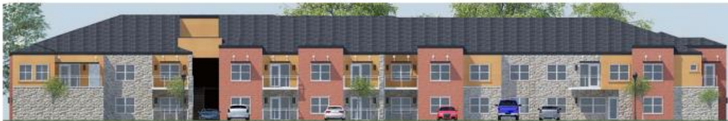
North Elevation - 76% Masonry (32% Brick, 44% Stone, 24% Stucco)
