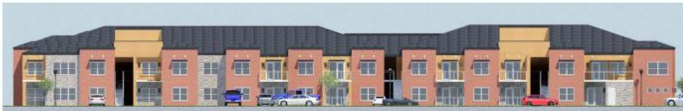
East Elevation - 78% Masonry (57% Brick, 21% Stone, 22% Stucco)
