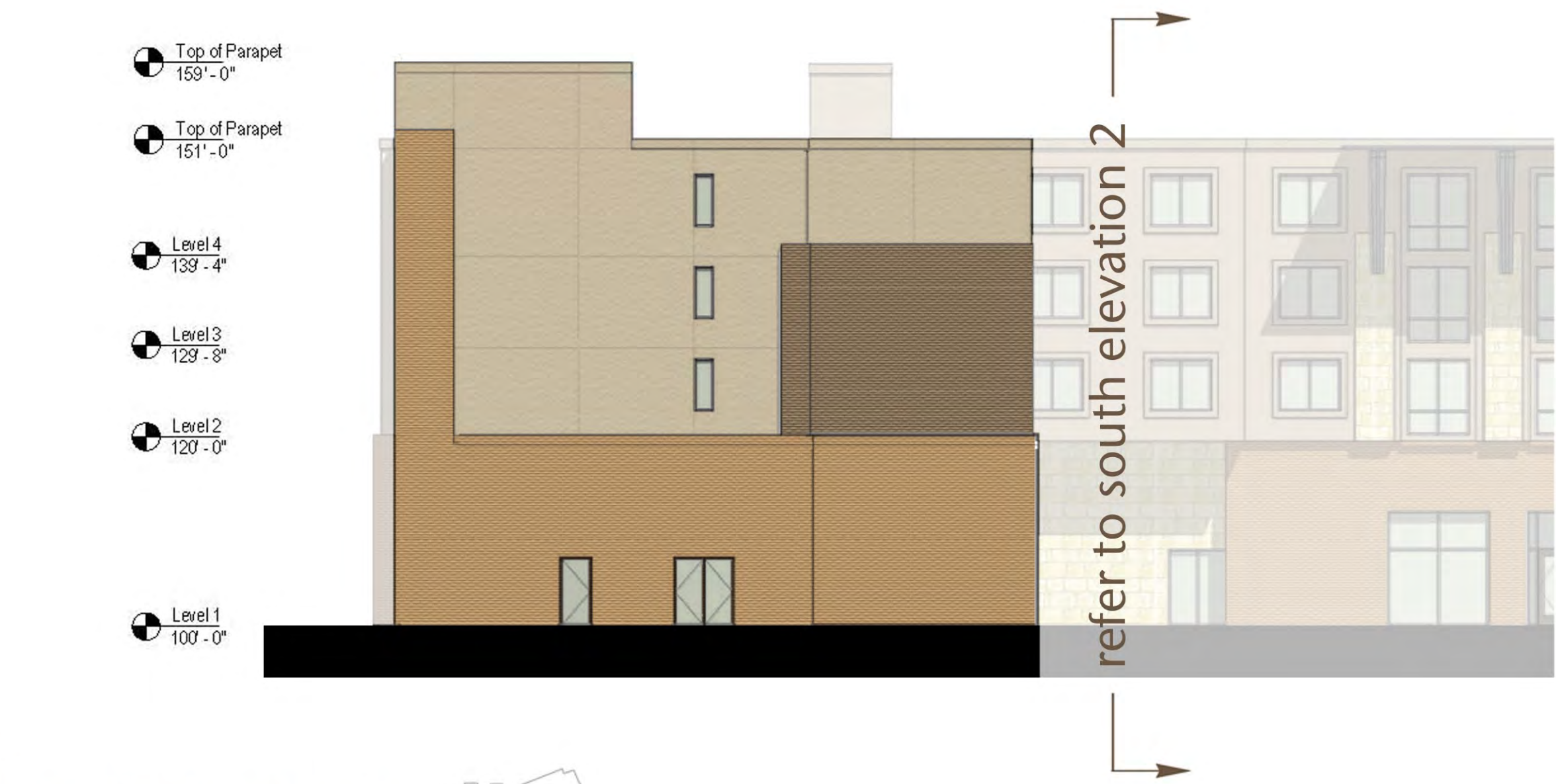
south elevation 1 52.4% masonry
