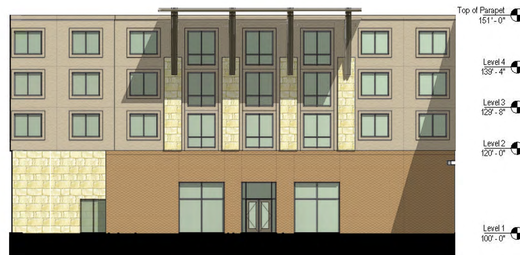
south elevation 2 50.4% masonry
