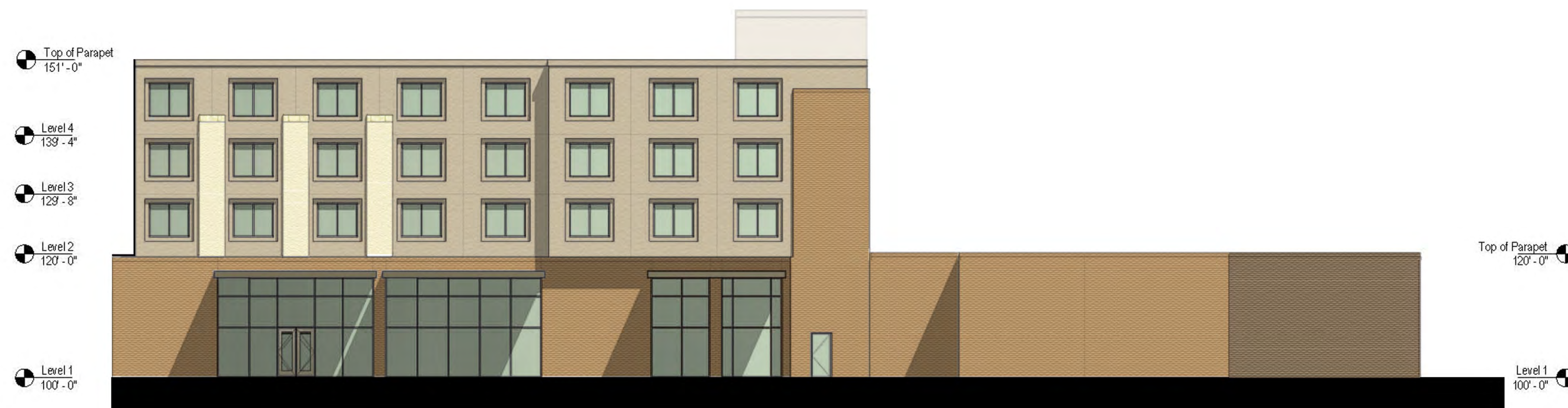
west elevation 2 52.7% masonry
