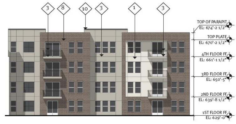
02 BLOCK A NORTH POOL COURTYARD ELEVATION
