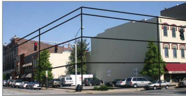
Figure showing how horizontal elements should match in the design of infill buildings.
