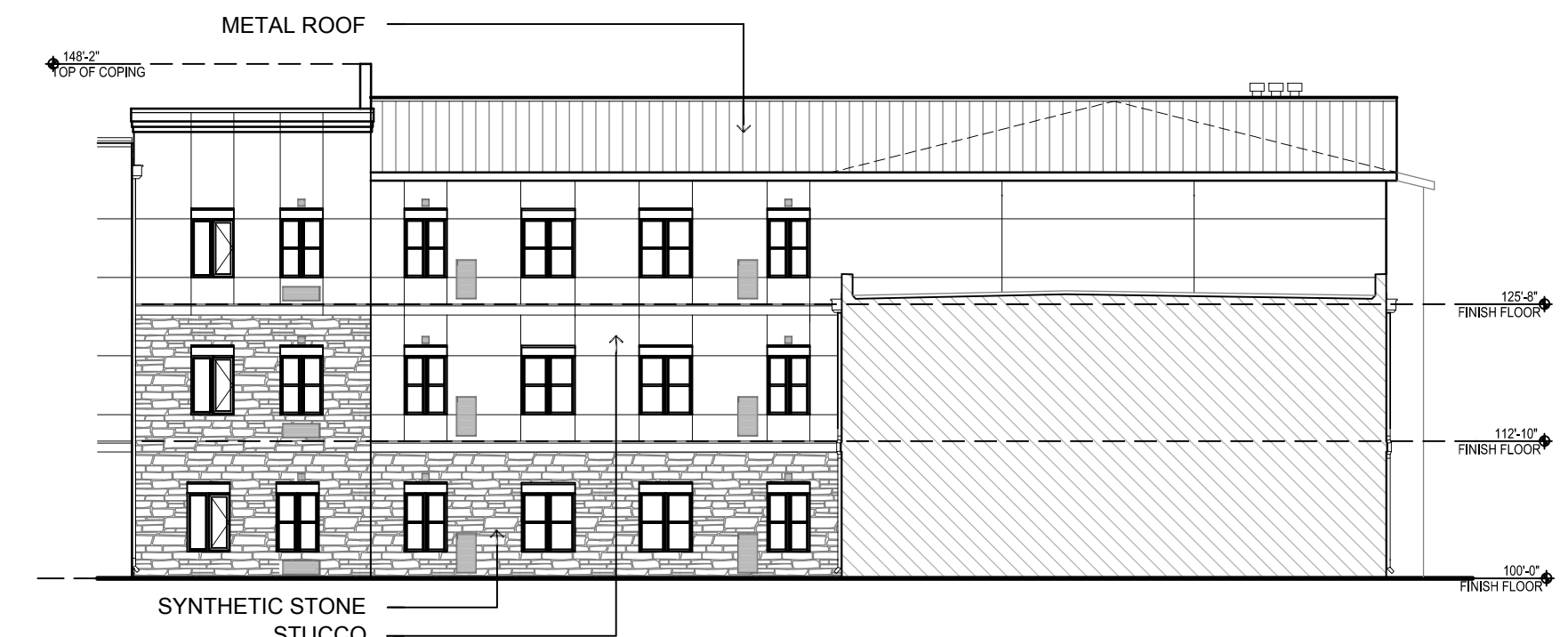
C4 BUILDING C-1 - NORTH ELEVATION 1/16" = 1'-0" STUCCO COVERAGE: APPROX. 1,804 S.F. SYNTHETIC STONE COVERAGE: APPROX. 852 S.F.
