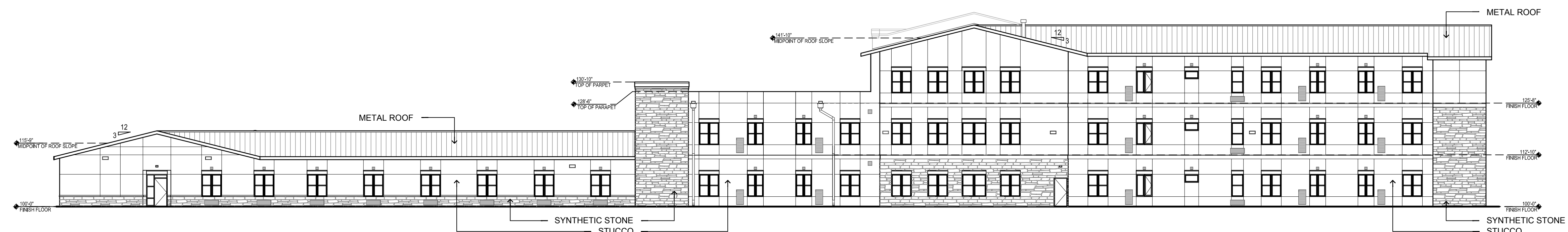
B1 BUILDINGS C-1 & C-2 - WEST ELEVATION 1/16" = 1'-0" STUCCO COVERAGE: APPROX. 6,414 S.F. SYNTHETIC STONE COVERAGE: APPROX. 1,814 S.F.
