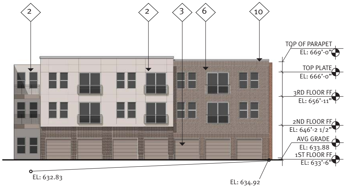
03 BLOCK B WEST ELEVATION (TENNESSEE ST)
