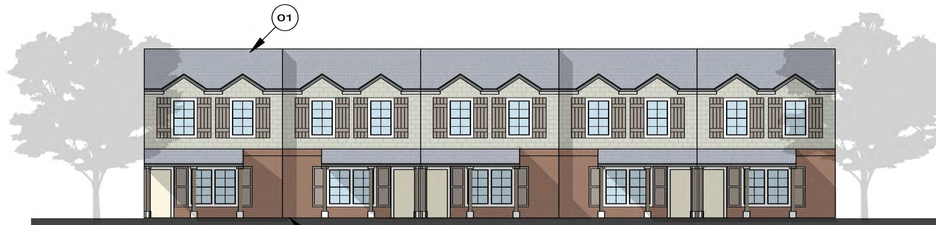
BUILDING #10 - NORTH ELEVATION BRICK: 50% (RED EARTH) STONE: 50% (AUSTIN WHITE) SYNTHETIC STONE: 0% (EARTH TONE MIXED) 5 10 15 20 25 20' 20' 20' 20' 20'
