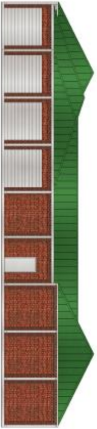
Building #2 West Elevation 100% Masonry (less Doors and Downspouts)
