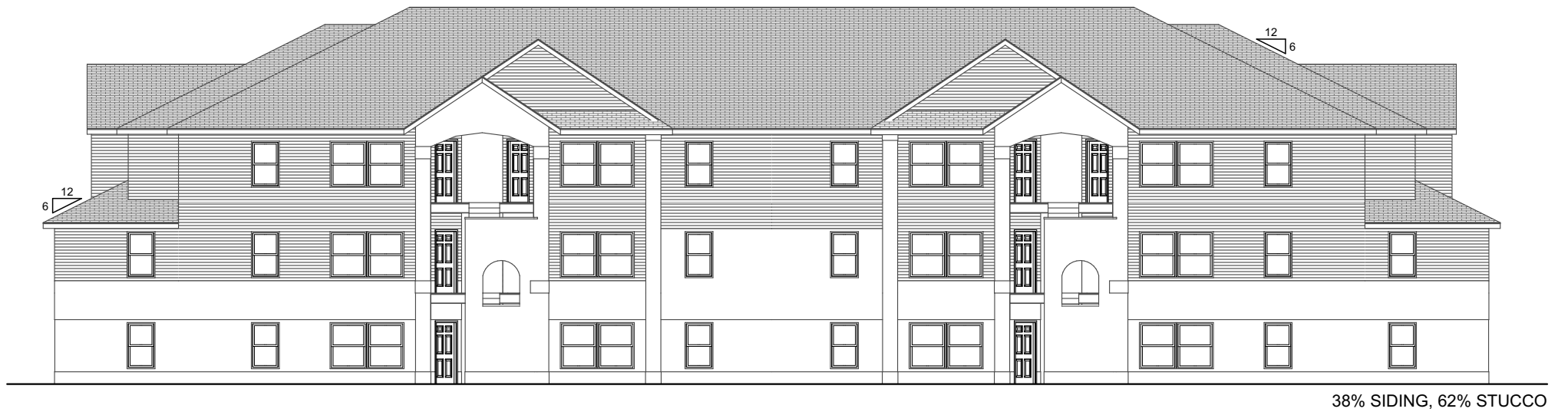
3 BLDG I REAR ELEVATION SCALE: 1/16" = 1'-0"
