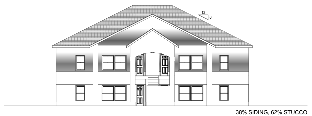
3 BLDG IV REAR ELEVATION SCALE: 1/16" = 1'-0" 0 8' 16' 32'
