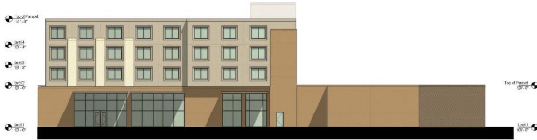
west elevation 2 52.7% masonry
