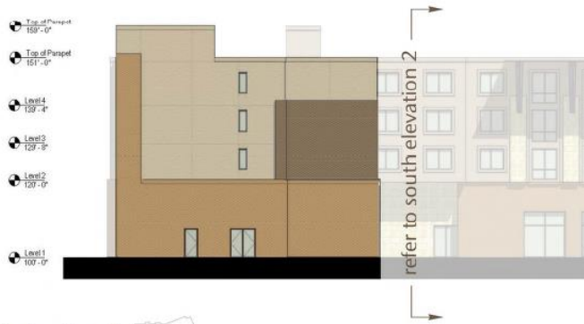
south elevation 1 52.4% masonry
