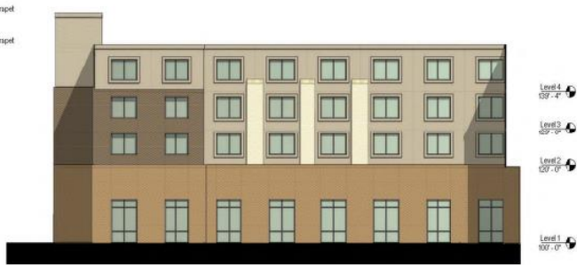
east elevation 2 53.2% masonry
