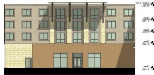
south elevation 2 50.4% masonry
