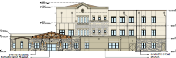
A3 BUILDING A - EAST ELEVATION
