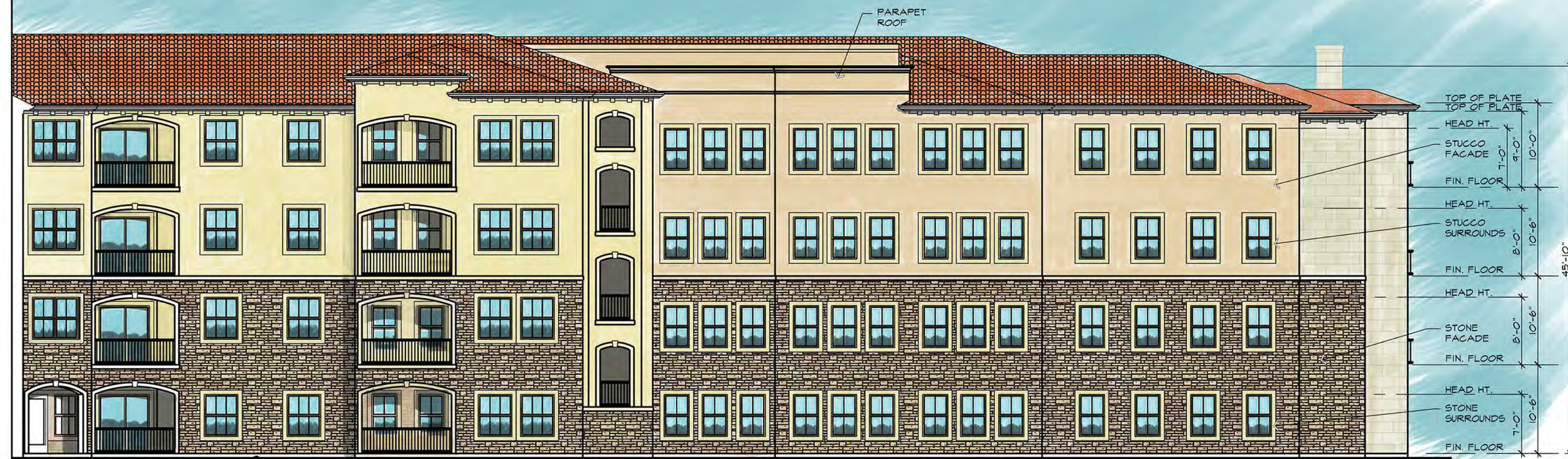
03 East Elevation- Office Wing SCALE: 3/32" = 1'-0"
