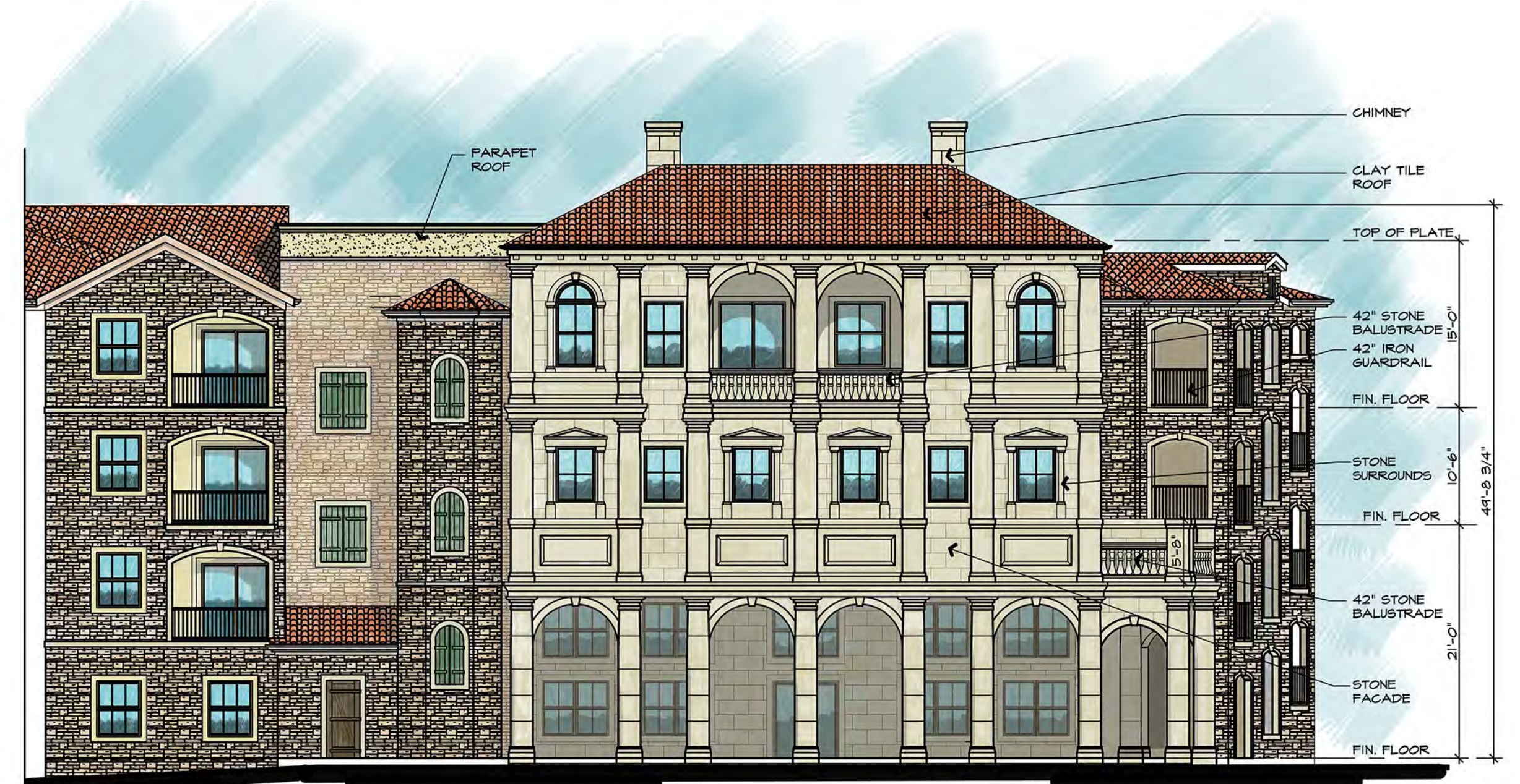
02 North Elevation- Entry SCALE: 3/32" = 1'-0"
