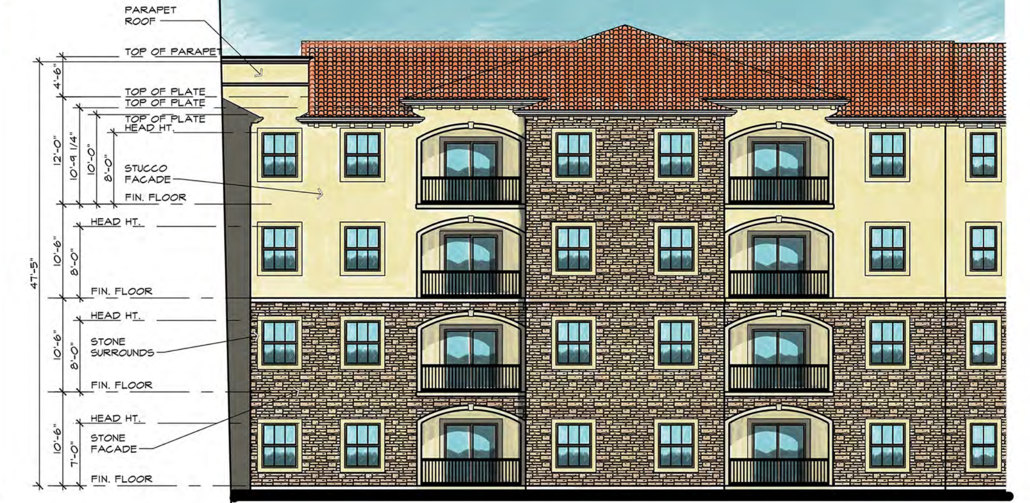
04 West Elevation- Courtyard SCALE: 3/32" = 1'-0"
