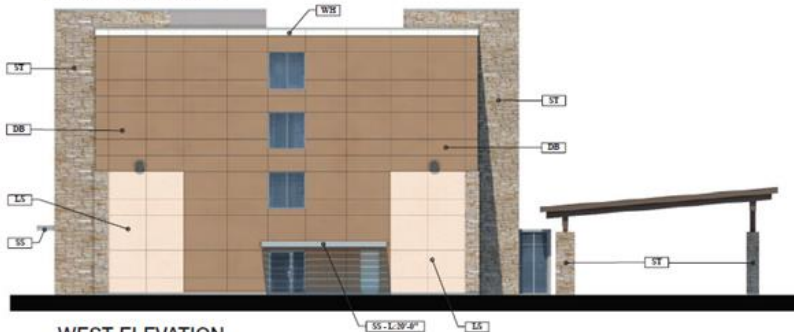
WEST ELEVATION 23.3% STONE TO STUCCO RATIO 13.5% WINDOW TO SURFACE RATIO
