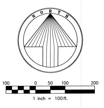
Basis of bearing, horizontal and vertical position derived from the Texas WDS RTK Network—Texas State Plane Coordinate System, NAD83, North Central Zone (4202).
