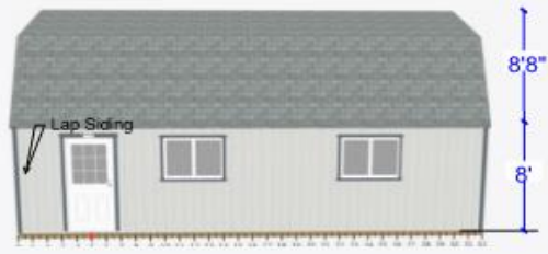
EAST ELEVATION Scale 1/4"=1'0" Lap siding =100% *Elevation color: Pastel Blue=95% *Accent Color: Royal Blue=5%
