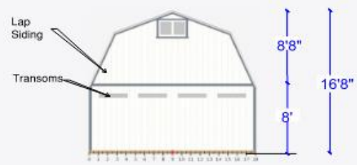
NORTH ELEVATION Scale 1/4"=1'0" Lap siding =100% *Elevation color: Pastel Blue = 95 % *Accent Color: Royal Blue = 5%
