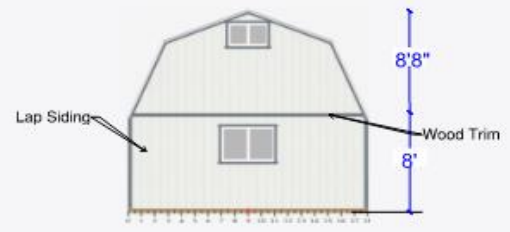
SOUTH ELEVATION Scale 1/4"=1'0" Lap siding =100% *Elevation color: Pastel Blue=92 % *Accent Color: Royal Blue=8%
