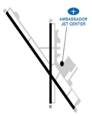
3,800 feet in length and 150 feet wide in good condition, while Runway 13/31 which is 6,451 feet long and 150 feet wide. The airfield has an ILS approach on Runway 31 and 4-Light PAPI on 13. Runway 13/31 has a weight limit of 110,000 pounds double tandem. This runway will accommodate most corporate aircraft in the small to larger range including G-V type aircraft. The
