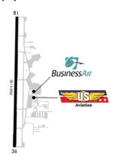
transient aircraft, the Airport maintains one asphalt/grooved runway in fair condition. Runway 18/36 is 150 feet wide and 7,002 feet in length. The single runway has a weight bearing capacity of 100,000 pounds double wheel and contains a precision ILS and a 4-light PAPI visual slope indicator on runway 18. This runway is capable of handling corporate aircraft up to a Gulfstream-V (G-V) category aircraft, which has a typical max takeoff weight of approximately 90,000 lbs.
