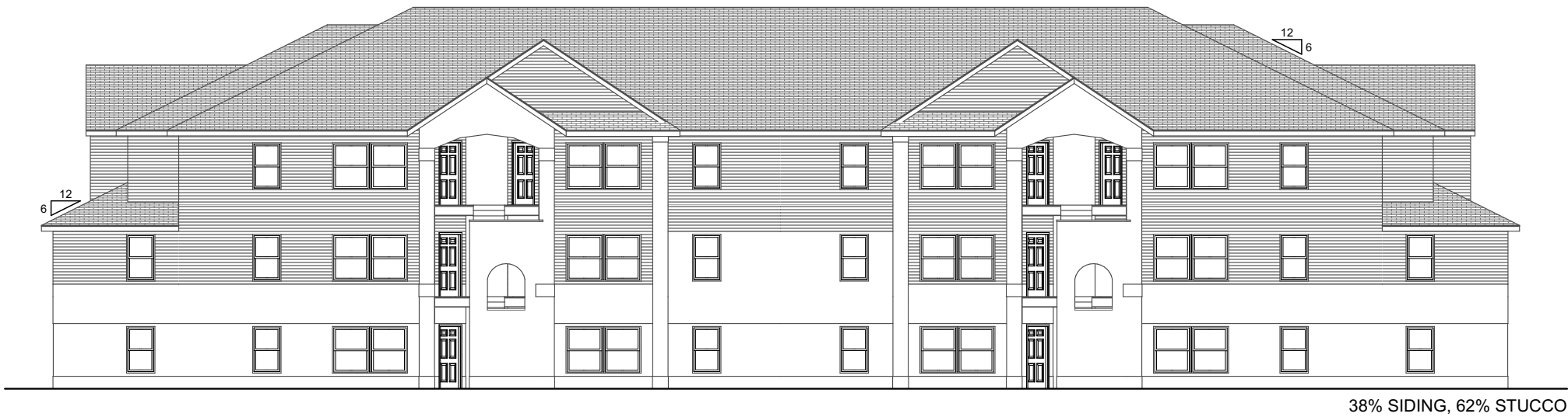
3 BLDG I REAR ELEVATION SCALE: 1/16" = 1'-0" 0 8' 16' 32'
