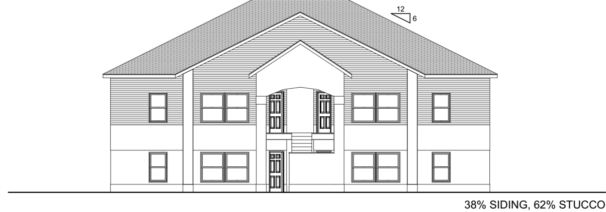
3 BLDG IV REAR ELEVATION SCALE: 1/16" = 1'-0" 0 8' 16' 32'
