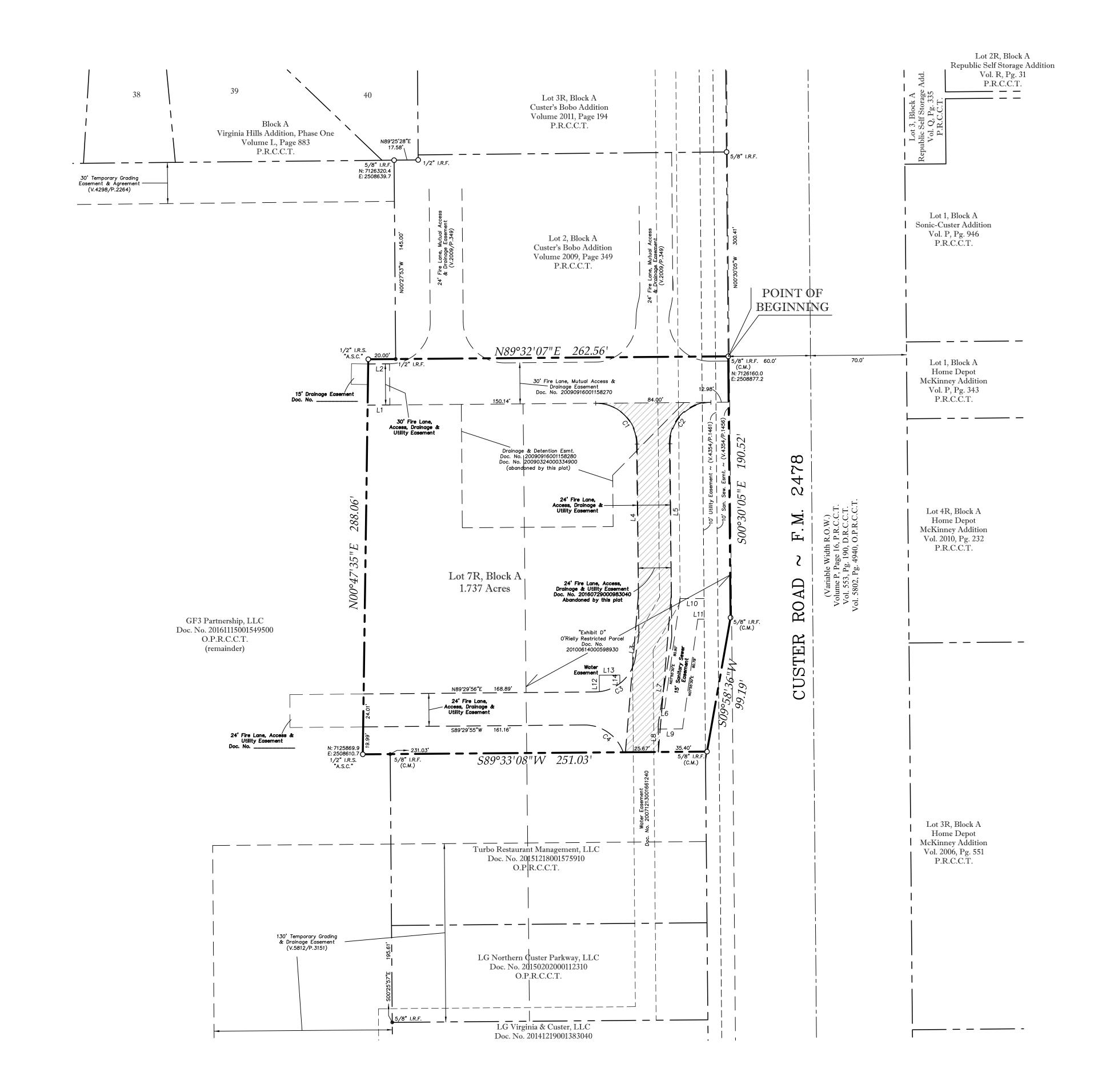
IRF - IRON ROD FOUND IRS - IRON ROD SET ROW - RIGHT-OF-WAY CM - CONTROL MONUMENT ASC - ARTHUR SURVEYING COMPANY WF - WATER FASEMENT PRCCT - PLAT RECORDS, COLLIN COUNTY, TEXAS RPRCCT - REAL PROPERTY RECORDS, COLLIN COUNTY, TEXAS ESMT - EASEMENT UTIL - UTILITY DRNG - DRAINAGE
