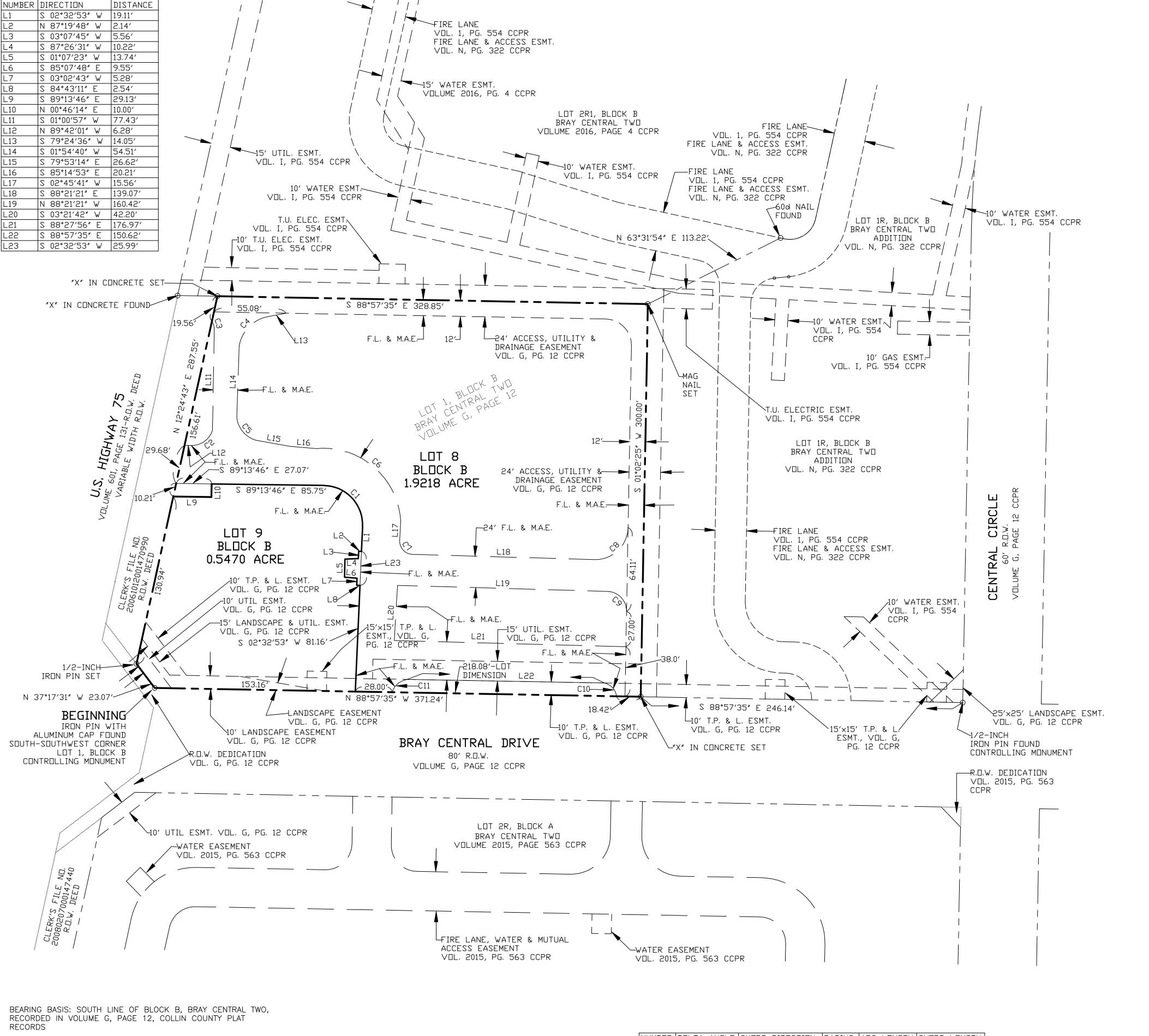
CONTROLLING MONUMENTS: 1/2-INCH IRON PIN FOUND AT SOUTHEAST CORNER OF SAID BLOCK B AND IRON PIN FOUND WITH ALUMINUM CAP FOUND AT SOUTH-SOUTHWEST CORNER OF SAID BLOCK B OF BRAY CENTRAL TWO.
