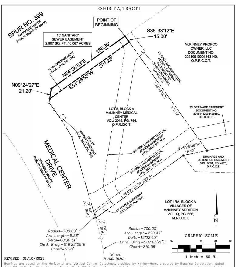
Bearings are based on the Horizontal and Vertical Control Datasheet, provided by Kimley—Horn, prepared by Baseline Corporation, dated June 02, 2015, for State Highway No. 5 (Cont. 0047; Sect. 04; Job 022). All coordinates shown are surface and may be converted to grid by dividing by a combined scale adjustment factor of 1.000152710. The survey plat shown herein is accompanied by a metes and bounds description of even date.
