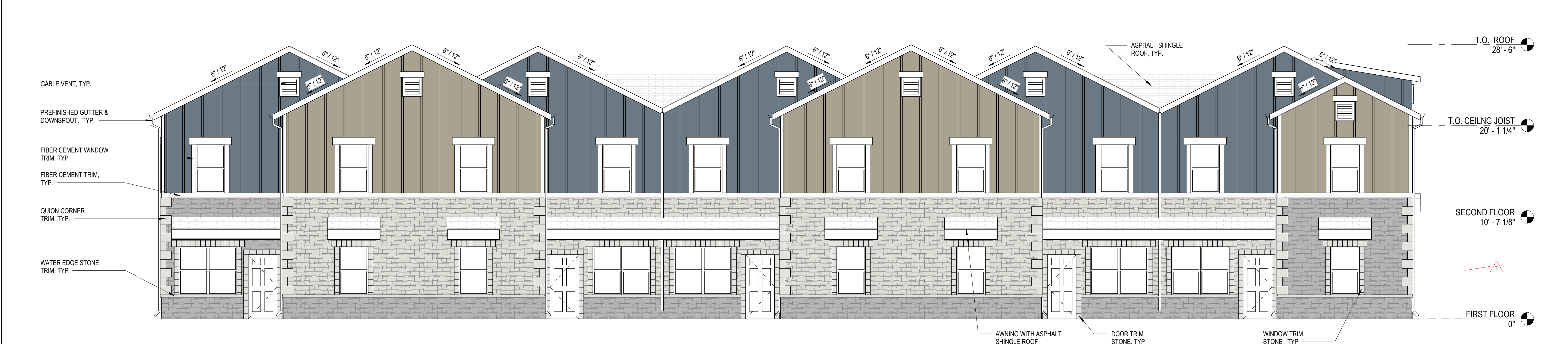
1 BLDG E - EXTERIOR ELEVATION 1 SCALE: 3/16" = 1'-0"
