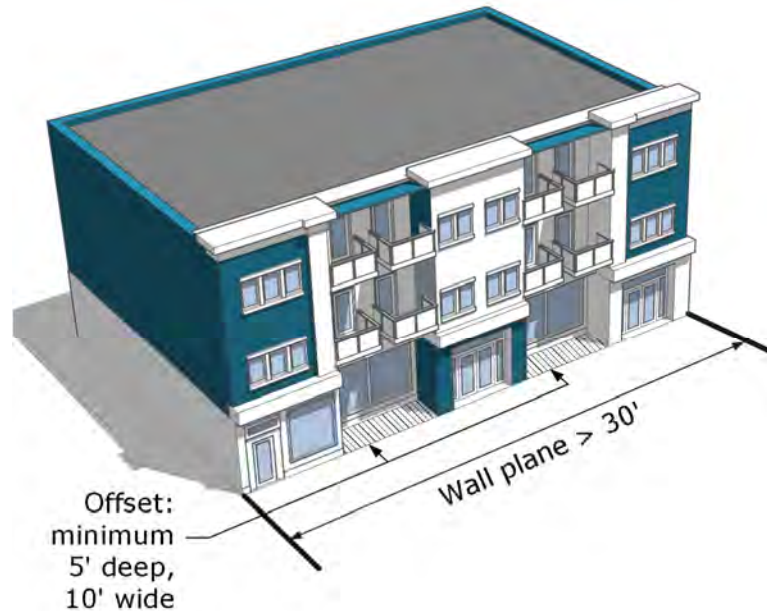
Figure 2-2932: Multi-Family Building Massing
