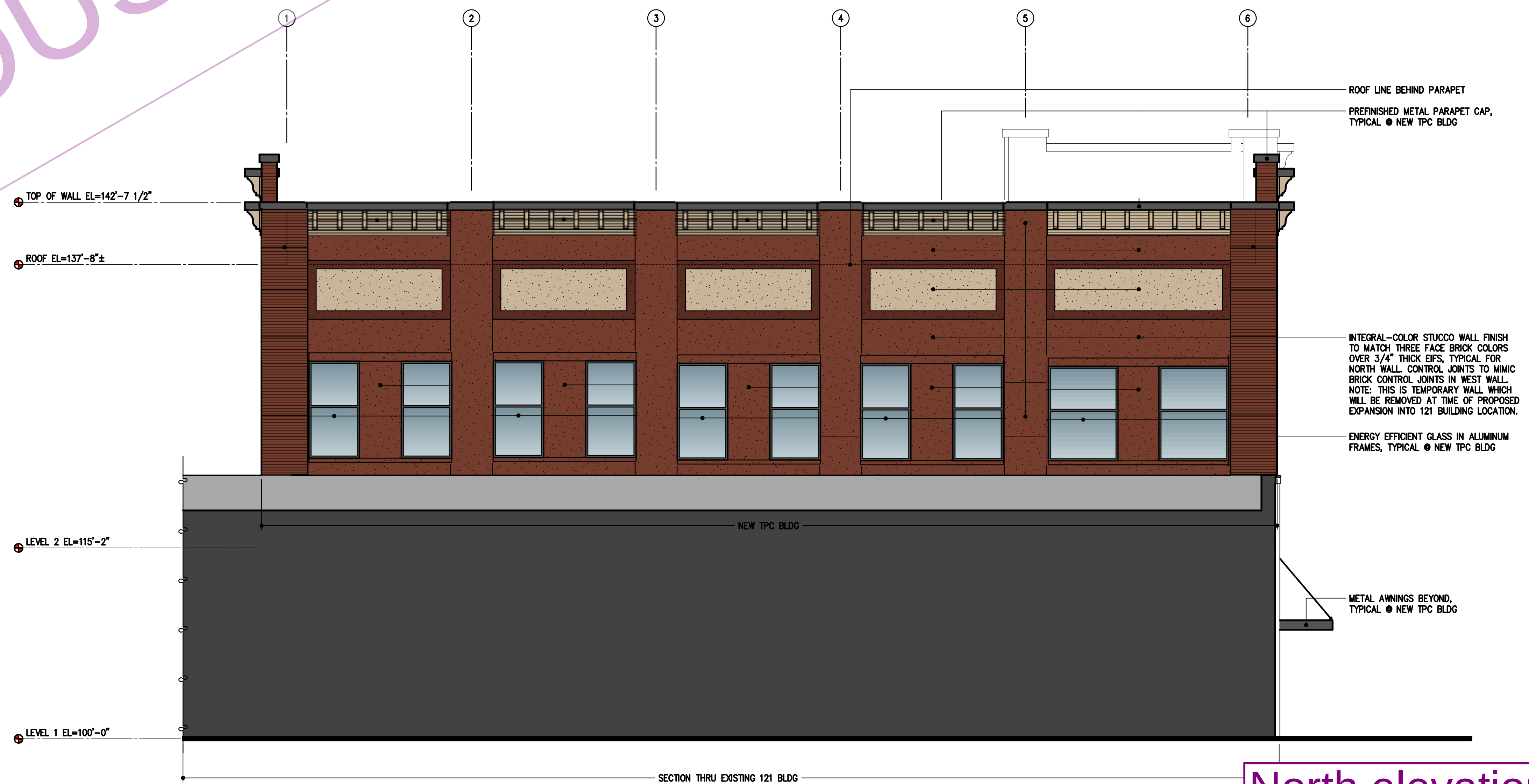
2 PROPOSED NORTH EXTERIOR ELEVATION 3/16" = 1'-0"
