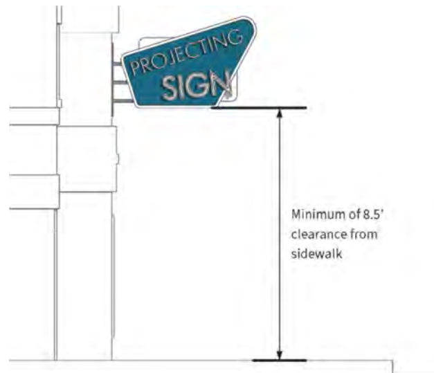
Figure 5-3: Projecting Sign Clearance
