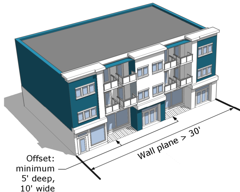
Figure 2-29: Multi-Family Building Massing
