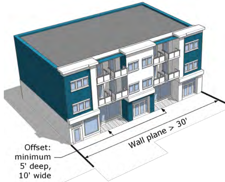
Figure 2-29: Multi-Family Building Massing
