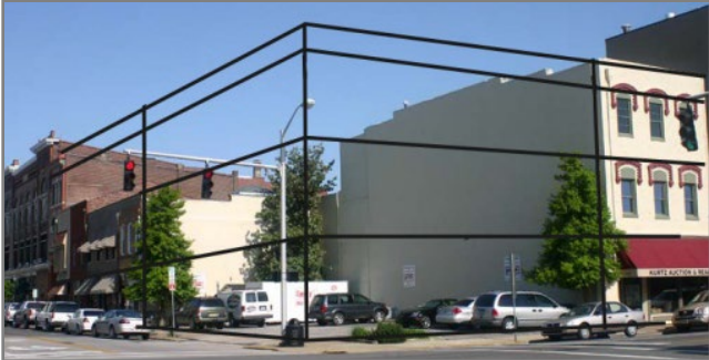
Figure showing how horizontal elements should match in the design of infill buildings.
