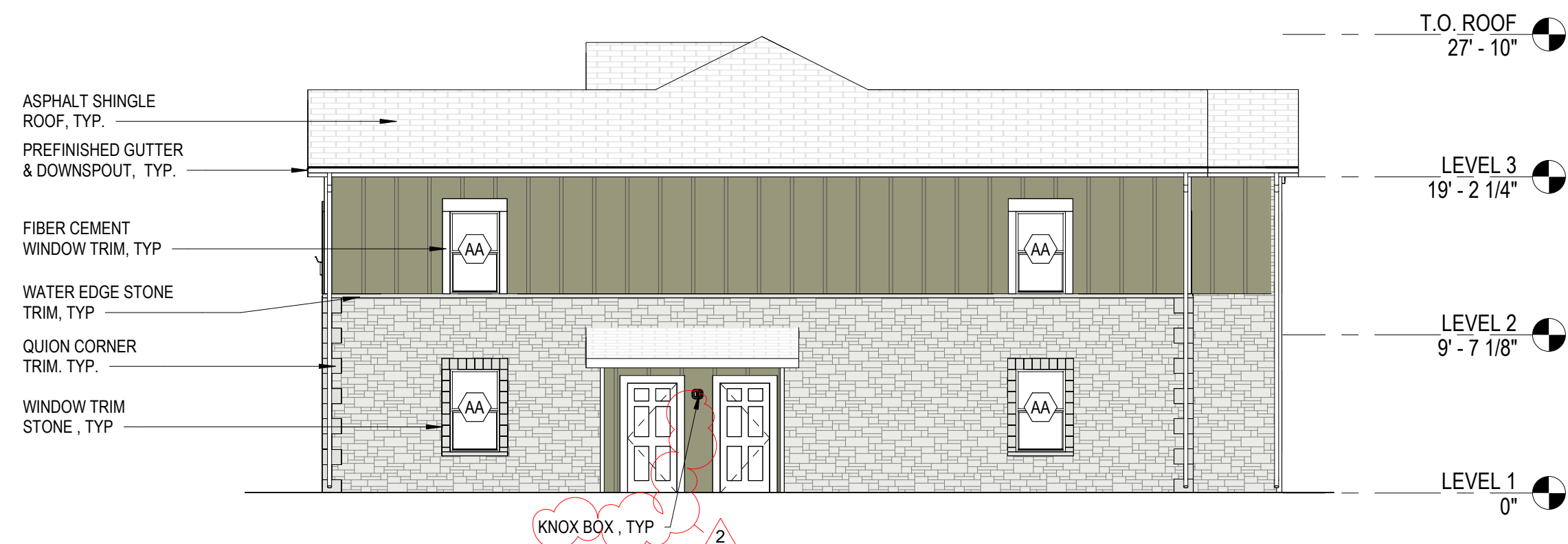
3 BLDG D - NORTH ELEVATION SCALE: 1/8" = 1'-0" REF: 1/A1.06
