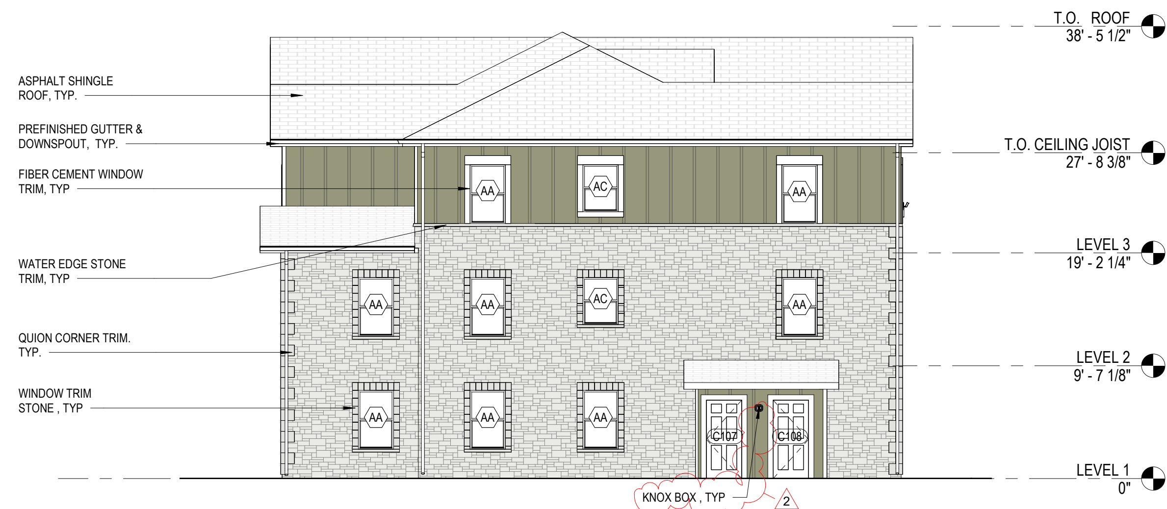
4 BLDG C - WEST ELEVATION SCALE: 1/8" = 1'-0"
